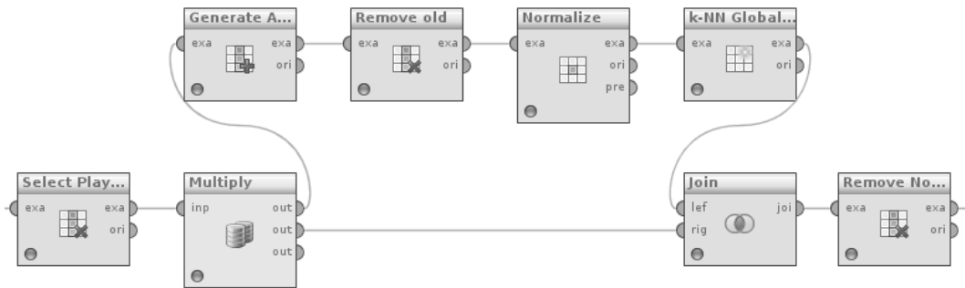
FIGURE 23.16: Processing the NBA data: Selecting important attributes, keeping a copy of the (not yet normalized data), normalizing the data and generating a data view, applying k-NN anomaly detection, and finally merging the outlier score back to the original data.
